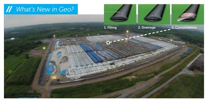
Figure 1. View of stacked geotextile tubes for containment of dredged sediments showing detail of multiple tube operation stages. (Photo courtesy of TenCate Geosynthetics.)
