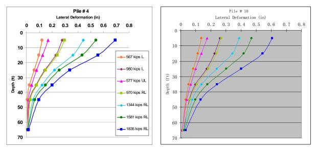
Figure 6. Profiles of Lateral Deformation for Piles 4 and 10 with Load Increments
