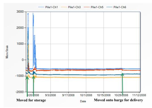
Figure 4. Recorded Strain Change for Pile 1 during Storage and Delivery
