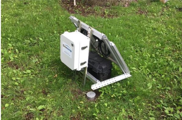
Example solar-powered seismograph
