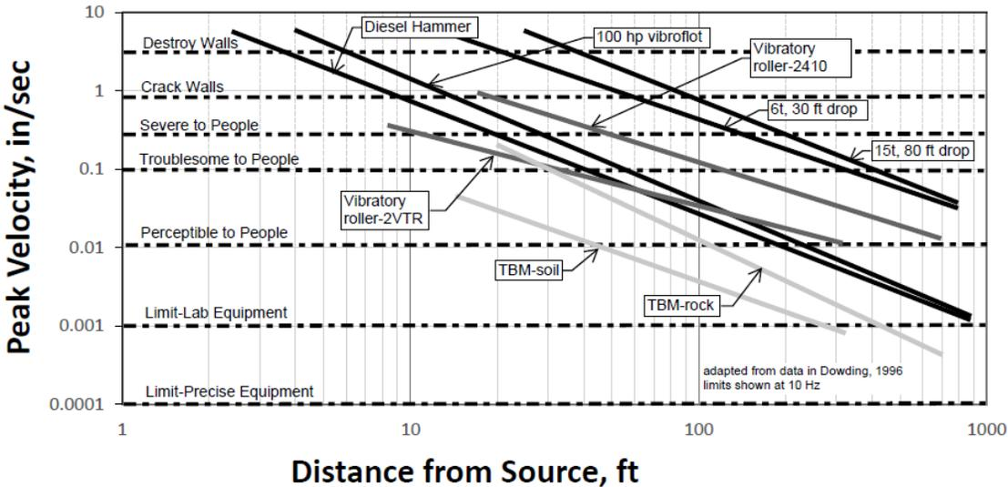
Figure 1 Typical ranges of measured PPV vs. distance for various construction equipment
