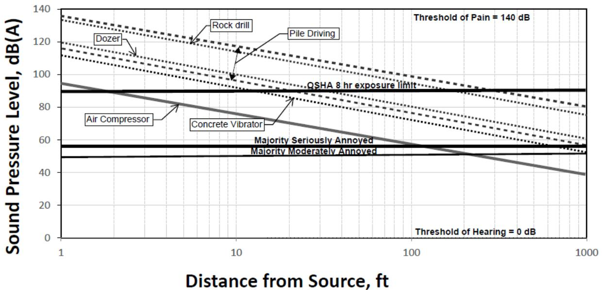
Figure 2 Typical ranges of measured sound pressure level vs. distance for various construction equipment
