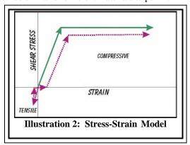
The analyses used the bilinear Mohr Coulomb strain-softening model with the parameters given in Table 9:
