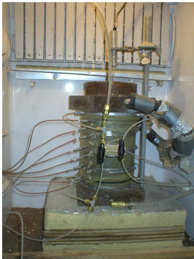
FIGURE 4— entire freeze-thaw / gas permeability test apparatus.
